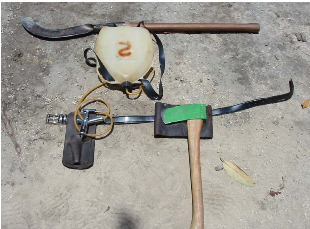
Image 8: Equipment typically used for pond apple control. From top to bottom: brush hook, 2.5 litre backpack, 5 millimetre "Phillips" injector gun, leather belt with holsters and "Tordon axe".
